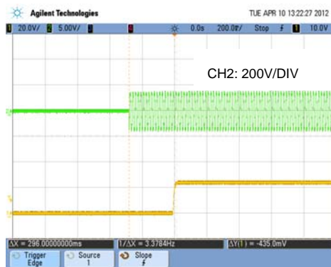
Vin=220VAC, Vo=24V @1.25A , At 25°C
