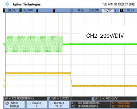
Vin=220VAC, Vo=24V @1.25A , At 25°C
