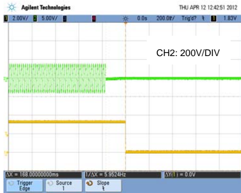
Vin=220VAC, Vo=3.3V @6A , At 25°C
