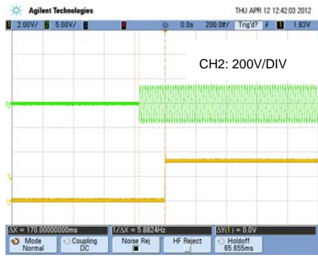
Vin=220VAC, Vo=3.3V @6A , At 25°C
